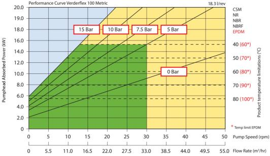
Displacement 18.3 l/revolution, Capacity is speed x 1.1 in m³/hr Minimum starting torque required: 4500 Nm Maximum peak power +28%
