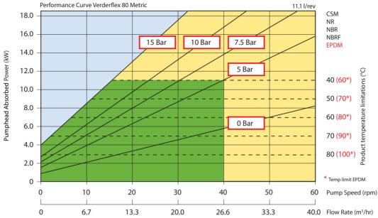
Displacement 11.1 l/revolution, Capacity is speed x 0.67 in  $m^3/hr$  Minimum starting torque required: 2000 Nm Maximum peak power +9%
