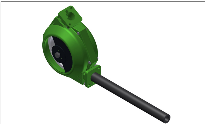
Figure 7 Installing the pump hose
